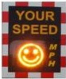
Croston and Heskin Parish Councils, a "Speed Indicator Device" (SID) which tells drivers if they are driving within the speed limit (a smiley face) or exceeding it (a glum face). Currently Bretherton only has the device for one month in three.
